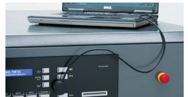
PC interface to simplify programming of wash cycles
